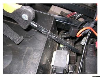
To the left you can see how I cut two slots for the wire entrance. Bending the cutout into a little ramp made a nice place to cable tie my wires.
