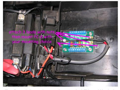
Then fasten it down using your chosen method. This could be dual lock strips, machine screws, or screws and nuts or even cable ties.
